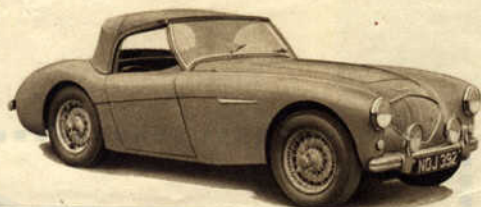
Showing the hood up: the centre-lock wire wheels are completely exposed, front and rear, and the length of the car is emphasized by a crease in the body panels.
